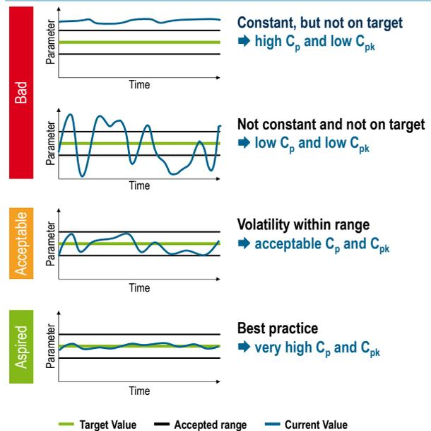
Figure 8: Illustration of  $C_p$  and  $C_{pk}$  – spread and deviation
